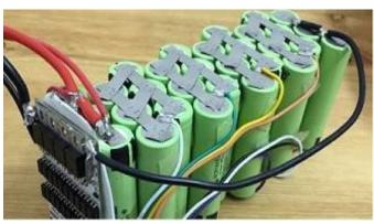
batteries, which are considered depleted when their capacity is reduced to 80%. While no longer suitable for mobile energy storage, these batteries could still have long lives in stationary settings. Second-life batteries can be used at utility-scale, commercial-scale, and even in community or local power applications....
